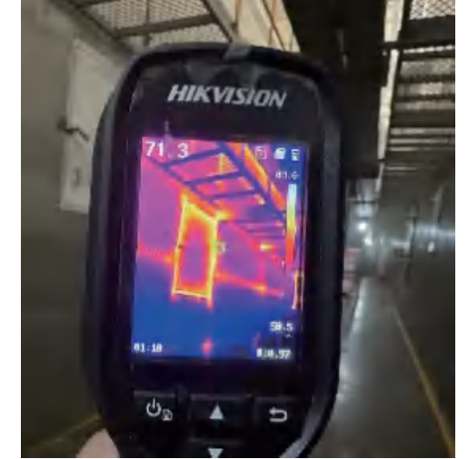
A thermal imager is used to check oven door tightness
